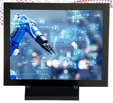
Densitron 15" rugged TFT with a resolution of 1024 x 768, optical bonded with PCT touch panel
